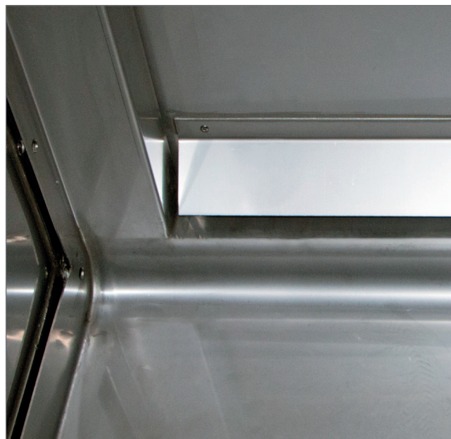
STRUCTURAL WORK WITHOUT SHARP CORNERS
